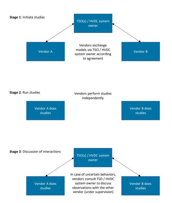
Figure 4-1: Workflow for Multi-Vendor interaction studies if vendors share data and models directly via the TSO(s) and / or HVDC system owner
