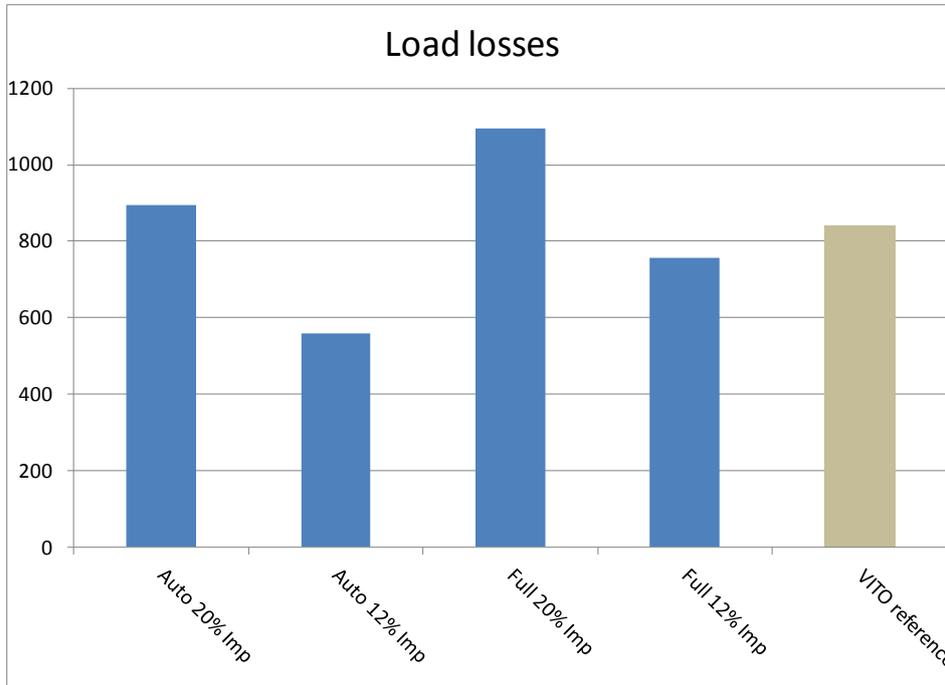
Fig. 2. Variation of load losses in four optimized transformers: Auto transformer 20 % impedance, Auto transformer 12% impedance, full transformer with 20% and 12% impedance respectively, compared to the VITO report reference power transformer
