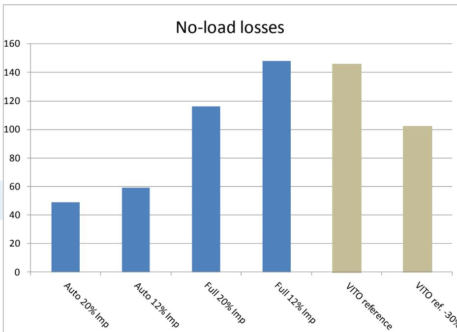
Fig. 1. Variation of no-load losses in four optimized 350 MVA 400/230 kV transformers from left: Auto transformer 20 % impedance, Auto transformer 12 % impedance, full transformer with 20% and 12 % impedance respectively. The VITO 350 MVA reference transformer and the VITO 30% loss reduced units are shown for reference.
